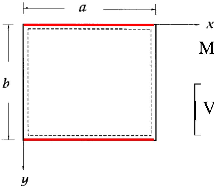
$$M_y = -D \cdot \left( \frac{\partial^2 w}{\partial y^2} + v \cdot \frac{\partial^2 w}{\partial x^2} \right)$$
