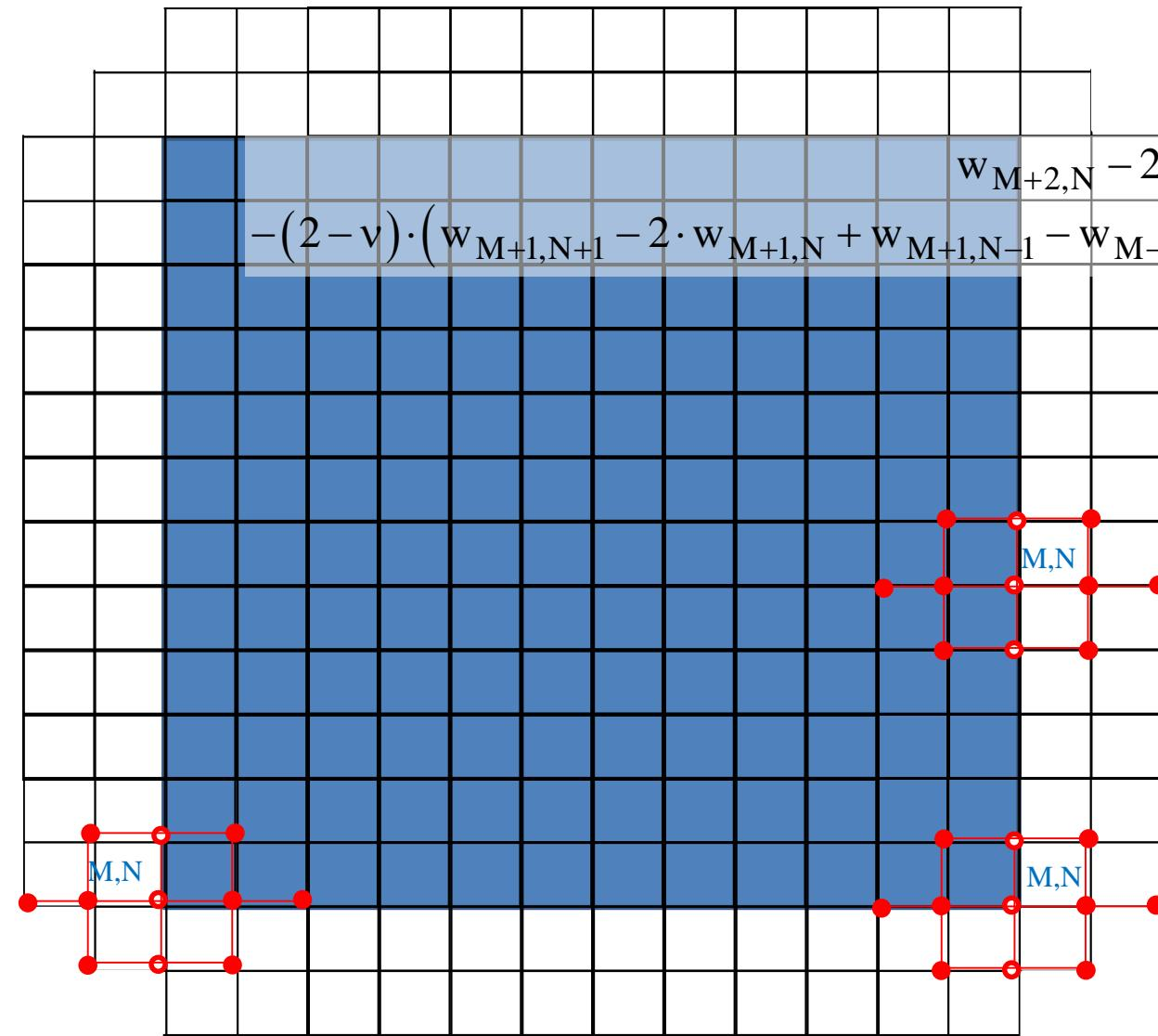
$$-D \cdot \left( \frac{\partial^3 w}{\partial x^3} - (2-v) \cdot \frac{\partial^3 w}{\partial x \partial y^2} \right)_{x=a} = 0$$
