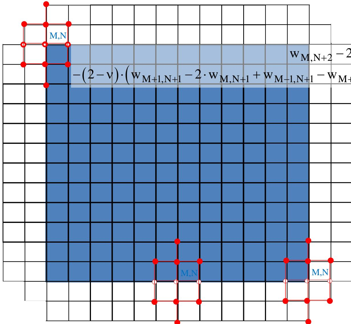
$$-D \cdot \left( \frac{\partial^3 w}{\partial y^3} - (2-\nu) \cdot \frac{\partial^3 w}{\partial x^2 \partial y} \right)_{y=b} = 0$$
