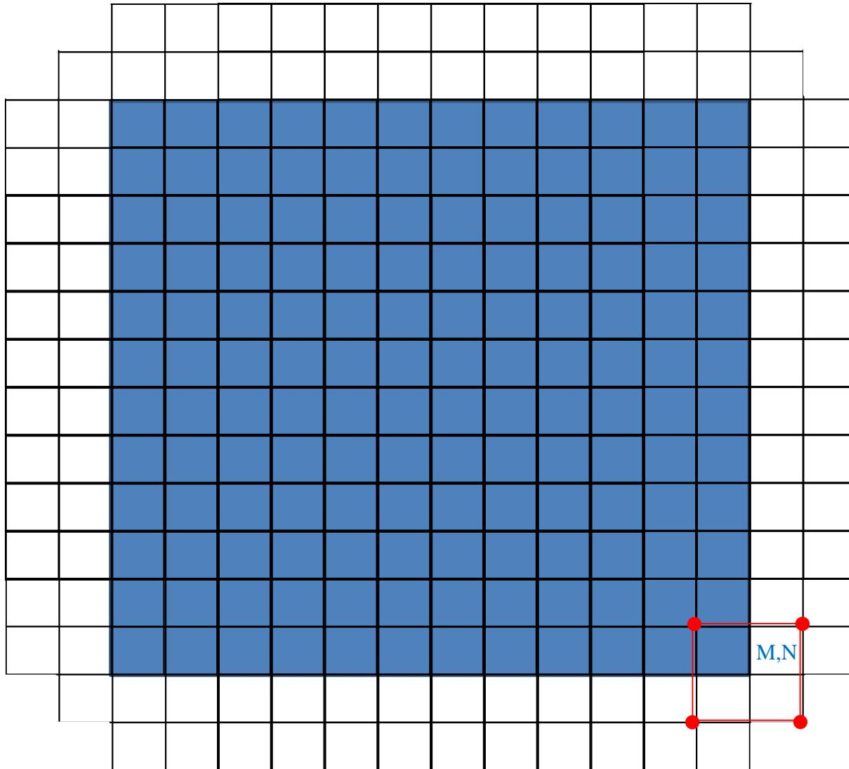
$$-(1-v) \cdot D \cdot \frac{\partial^2 w}{\partial x \partial y} \Big|_{\substack{x=a \\ y=b}} = 0$$
