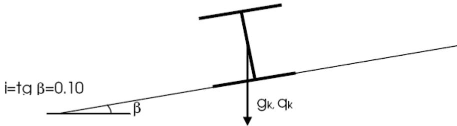
Homework 4: The beam-column represented in the figure below is loaded by an axial force  $N_k = 50$  kN and a transverse load whose permanent and variable parts are  $g_k = 3.0$  kN/m and  $q_k = 5.0$  kN/m, respectively.
